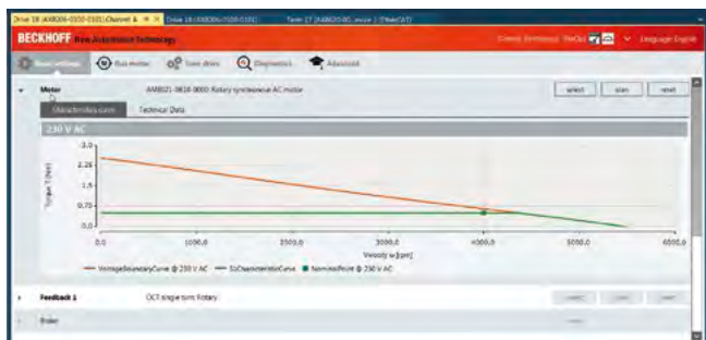
Detailed visualisation of the motor characteristic according to the electronic identification plate
