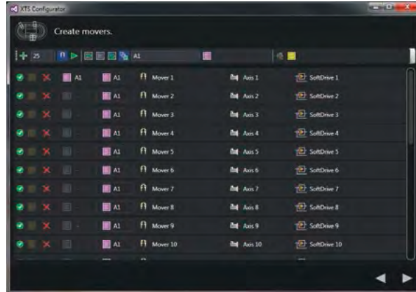
Axis and controller parameters of a mover can simply be copied within the XTS configurator.
