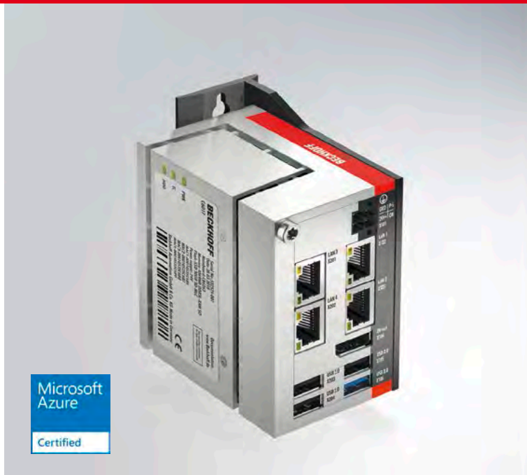
C6017 for installation at the rear wall
