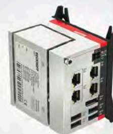
C6017 for installation at the side wall
