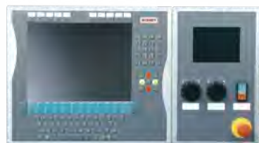
Extension with additional display, incremental encoders and switch elements
